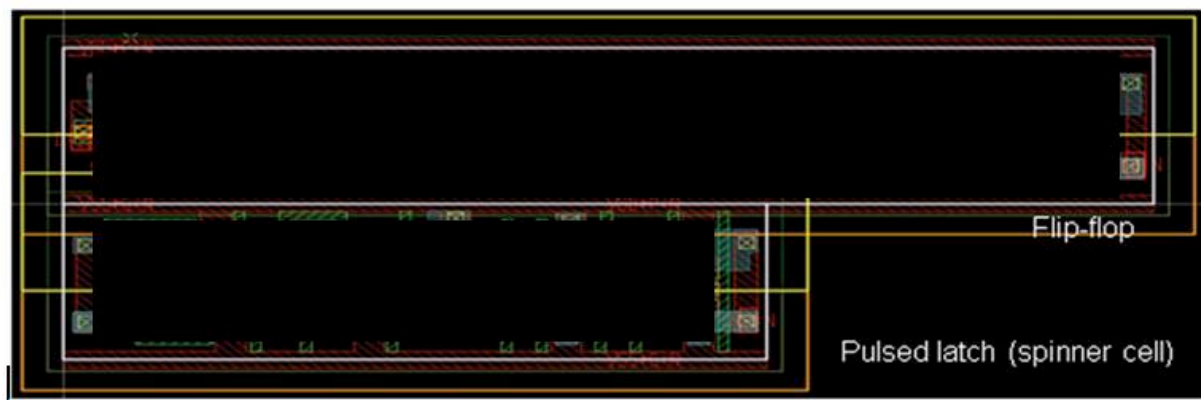
Figure 1: Flip-Flop and pulsed latch structures
