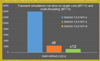
SMASH speed-up simulation gain thanks to new NICSLU solver and RC reduction method, with 335k capacitors, 32k MOS and 210k resistors
