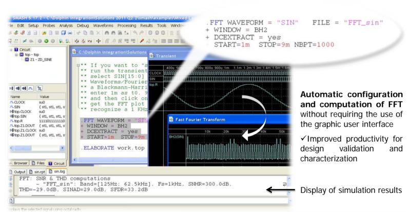
Dialog for user friendly configuration of FFT analysis on analog and logic signals
